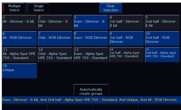
Groups window (on FLX) with various fixtures current selected highlighted in blue
