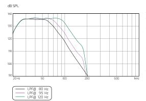
This graph shows the frequency response for a 1-watt swept sine signal in a semi-anechoic environement  $(2\pi)$ , measured at 3 m and scaled down at 1 m. In order to provide more precise information for acoustical analysis, a 1/6 octave smoothing has been applied.
