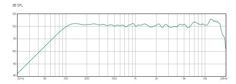
The above graph shows the frequency response for a 1-watt swept sine signal in an semi-anechoic environement  $(42\pi)$ , measured at 3 m and scaled down at 1 m.
