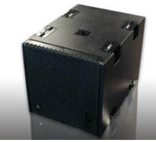
The Metrix convertible cardioid sub boasts two newly designed ND15-S 15" Neodymium Kevlar drivers specifically designed for the Metrix Sub. They are manifold mounted within an ultra compact, tuned, and vented enclosure. The Metrix Sub-t can be flown with both the i & t series and can be used as a pole mount base with a pair of Metrix W-t's. The Metrix Sub-i includes no rigging hardware and is designed for use in ground stacking applications only.
