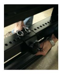
For the Install version of the rigging frame, attach the hanging bracket to the steel frame. Note that there are several positions alongside the middle bar to attain the desired frame angle when flown.
