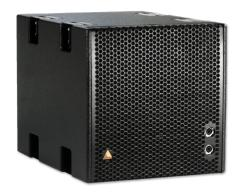
This ultra compact line array loudspeaker is a convertible cardioid sub; a single-sided box that can be arrayed conventionally or arrayed in back-to-front pairs for true cardioid performance. The Metrix Sub is equipped with two newly designed, powerful 15" ND15-S Kevlar neodymium bass drivers, mounted in a tuned, vented and fully braced cabinet.
