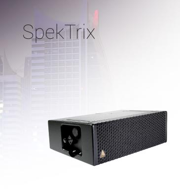
Designed for optimal ease-of-use, the Adamson SpekTrix is a three-way active loudspeaker that employs two dedicated 8" Kevlar neodymium drivers and one 1.4' exit high frequency compression driver mounted on a proprietary wave shaping sound chamber. SpekTrix offers a defined coverage pattern of 120° x 5° (H x V).
