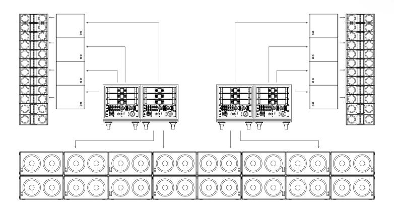
The SpekTrix High Performance set can be divided into two smaller systems. You can also expand the system as your company grows by adding 8 SPK and 8 SPB with your exsisting amps and racks.
