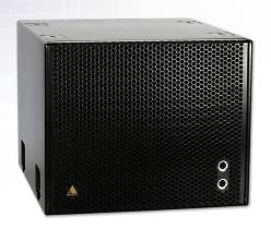
A compact sub-bass loudspeaker designed to provide high SPL low-end extension to SpekTrix line array loudspeakers. It is equipped with two powerful 18' Kevlar cone drivers in a tuned and vented enclosure. The SpekTrix Sub features convertible cardioid technology. It can be arrayed conventionally (all enclosures facing the same way) or in front-back or front-back-front setups for true cardioid performance.
