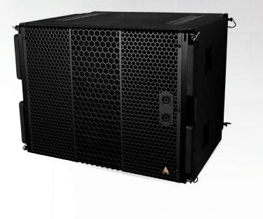
The S119 Subwoofer is the companion subwoofer to the S10. The enclosure is loaded with a light weight, long excursion, 19" ND19 Kevlar Neodymium driver utilizing Adamson's Advanced Cone Architecture and a 5" voice coil for exceptional power handling. It is mounted in an ultra-efficient front-loaded enclosure, designed to reproduce clean, musical low frequency information.
